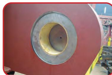
COM-KU®/D Bushings for double-stroke Hydraulic Cylinder, Split Hopper Barge
