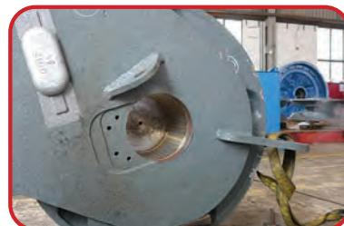
LUB-MET® Spherical Bearings GE 400 for Chain Stoppers
